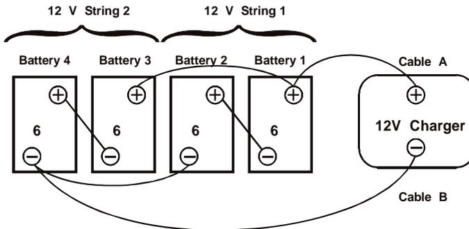
**Fig 3. Series-Parallel Connection**
