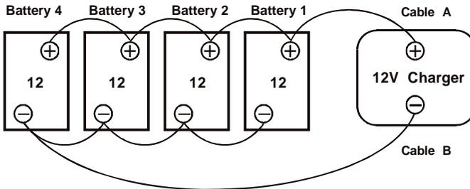
**Fig 2. Parallel Connection**
