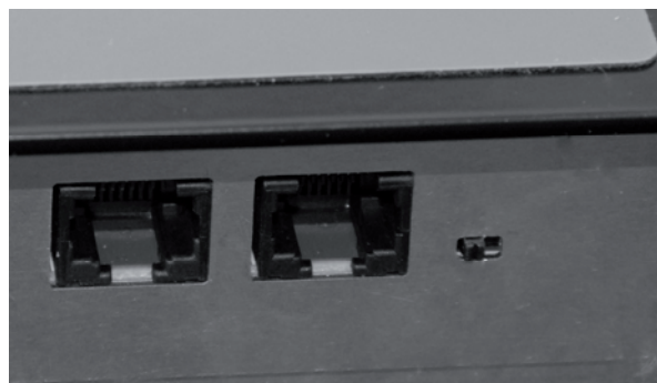
RCC-03 termination activated (left position)
