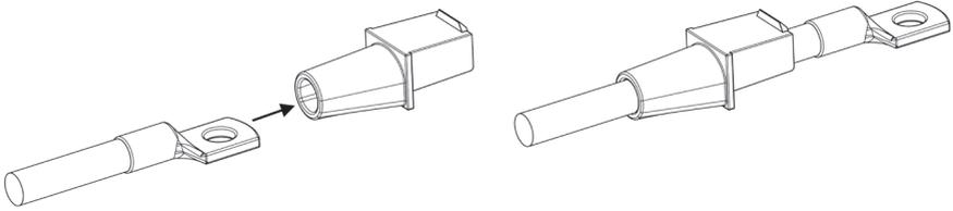
When the DC cables are connected to the charger, the rubber grommets can be slid towards the charger's front panel until the screw connections are completely covered.
