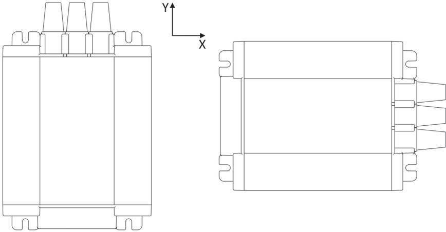
6. Use the base of the charger as a mounting template to mark the positions of the fixing screws.
