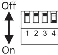
DIP switch 1 and 2 are used select the desired charge program for the connected output battery. Please see the table below:
