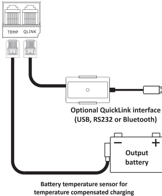
The optional QuickLink communication Kits allow the charger to be programmed and monitored using the Samlex Dashboard software on PC (via USB or RS232) or the Dashboard Mobile app on iOS and Android platforms (via Bluetooth).
