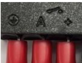
\* If you use your own switch, you must connect the switch between "A" and "+". Between "A" and ⊖ an LED or incandescent light can be used. Please note that an 12V LED / incandescent lamp is used. We can't guarantee the LED / incandescent lamp operates unless the switch in this set is used.
