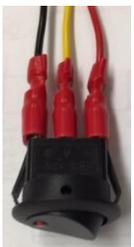
2.) Connect the smallest fastons to the switch
