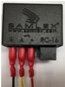
1.) Connect fastons to RC-16 unit: Use this side with the largest fastons
